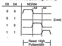
For output OROUT, (assuming A1 > A2 > A3 > A4), a variety of output waveforms can be produced, many of which will be the same as one or the other of the NOR outputs. This results from setting one of the NOR outputs to 'Low' with the (0,1) D-input combination so that OROUT is determined by the other NOR output, or from masking one NOR waveform with the
