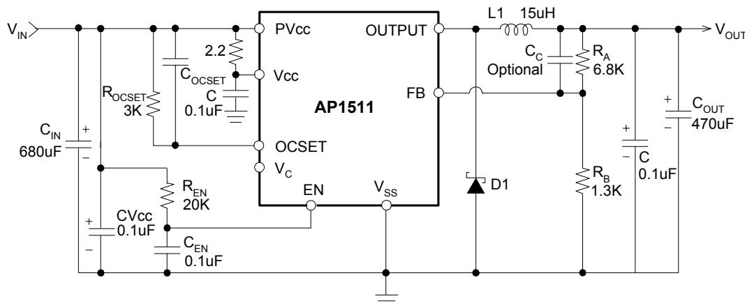
Note:  $V_{OUT} = V_{REF} \times (1 + R_A/R_B)$
