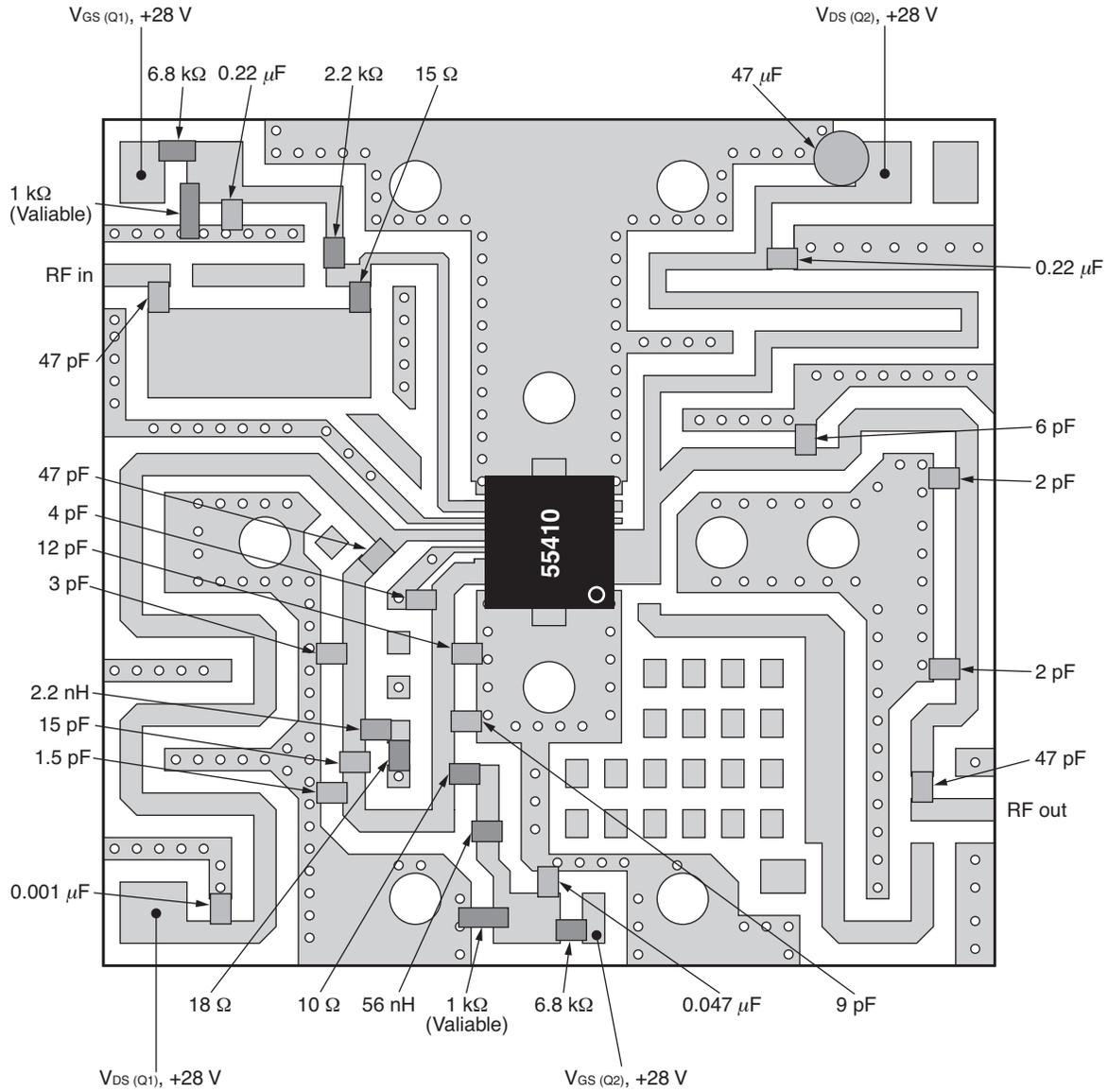
EVALUATION CIRCUIT (f = 2 090 to 2 190 MHz, V<sub>DS</sub> = 28 V, I<sub>Dset</sub> = 120 mA)
