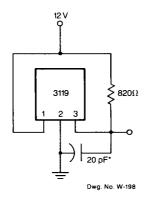
\*Includes probe and test fixture capacitance.
