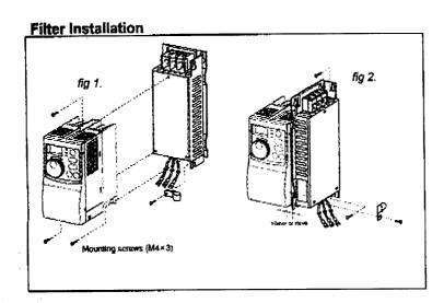
The filter can be attached using either a footprint (fig 1.) or a bookshelf (fig 2.)
