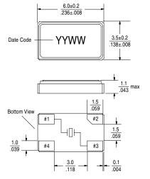
Pads #2 and #4 are connected to metal lid for shielding to minimize EMI
