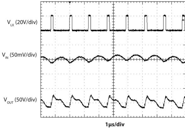
Typical Waveforms at  $V_{IN} = 5.5V$
