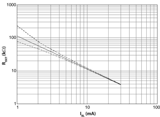
Figure 2 – Set Resistor Value Selection Graph
