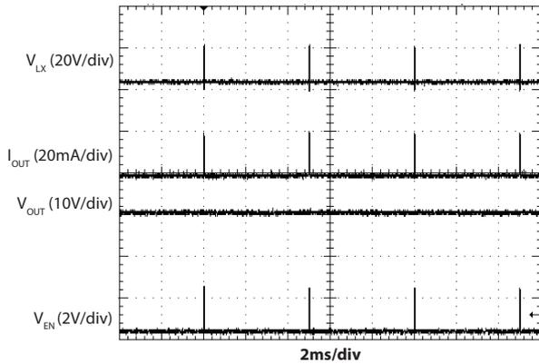
PWM Operation at 50kHz and 15% Duty Cycle
