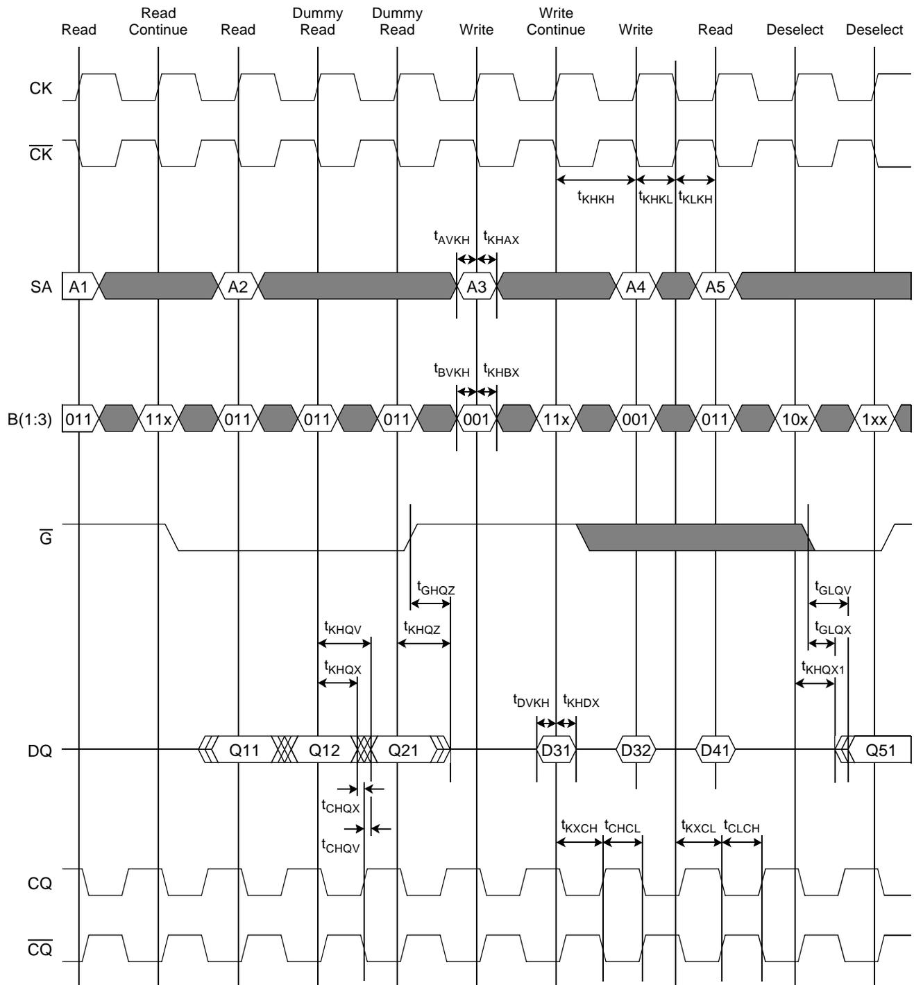
**Note:** In the diagram above, two Dummy Read operations are inserted between Read and Write operations to control the data bus transition from output to input. This depiction is for clarity purposes only. It is NOT a requirement. Depending on the application, one Dummy Read operation may be sufficient.
