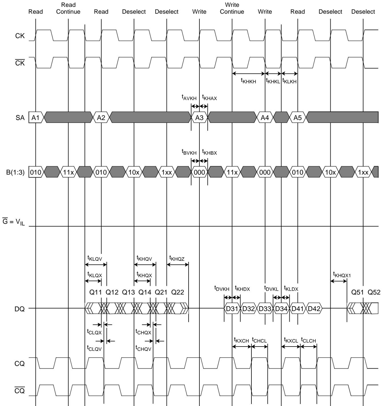
**Note:** In the diagram above, two Deselect operations are inserted between Read and Write operations to control the data bus transition from output to input. This depiction is for clarity purposes only. It is NOT a requirement. Depending on the application, one Deselect operation may be sufficient.
