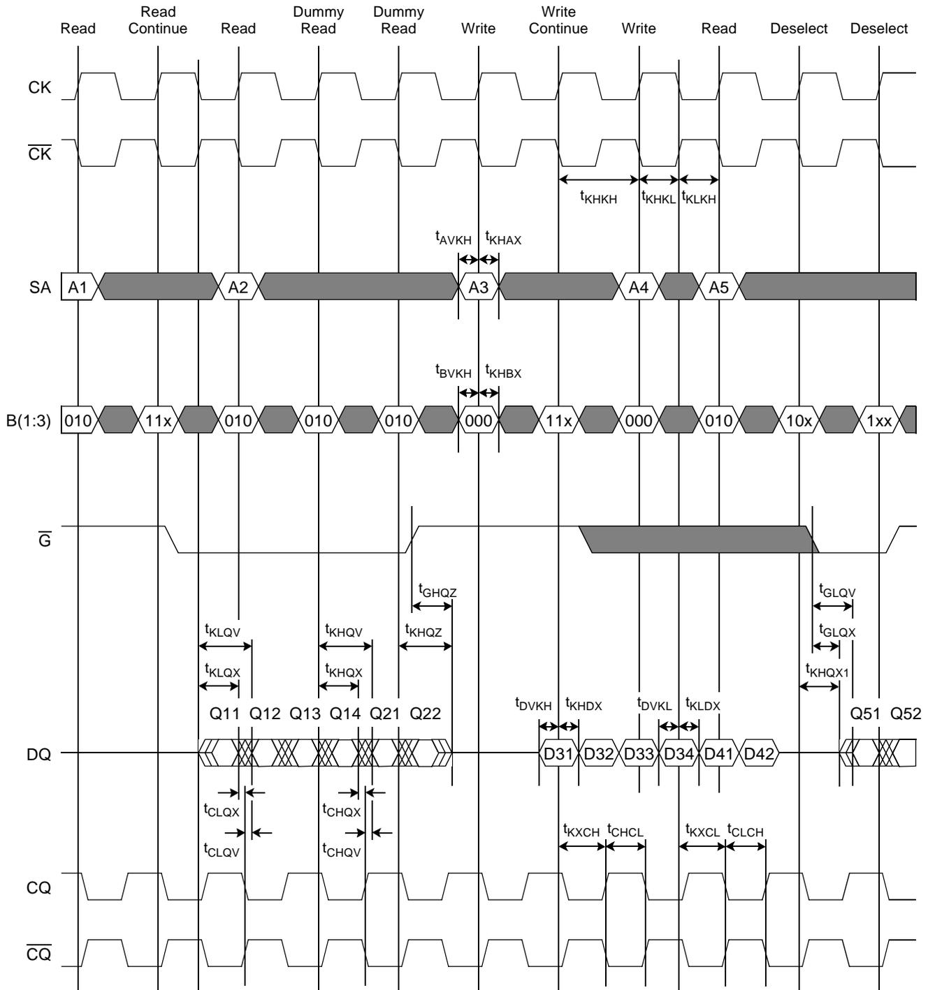
**Note:** In the diagram above, two Dummy Read operations are inserted between Read and Write operations to control the data bus transition from output to input. This depiction is for clarity purposes only. It is NOT a requirement. Depending on the application, one Dummy Read operation may be sufficient.
