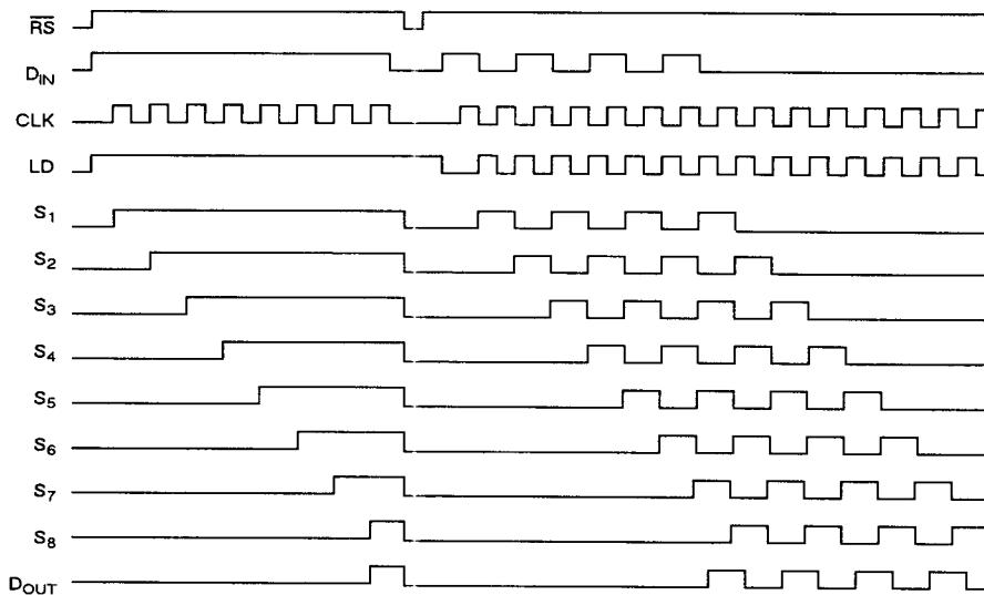
S<sub>1</sub>-S<sub>8</sub> and D<sub>OUT</sub> are expected output with the drain connected high.
