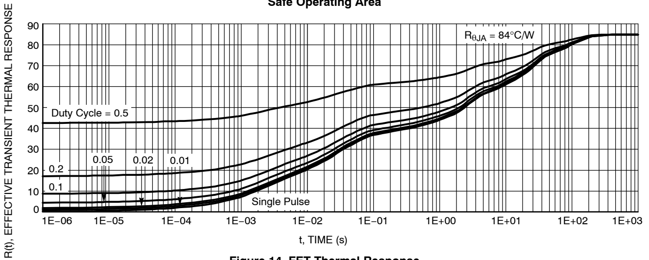
Figure 14. FET Thermal Response
