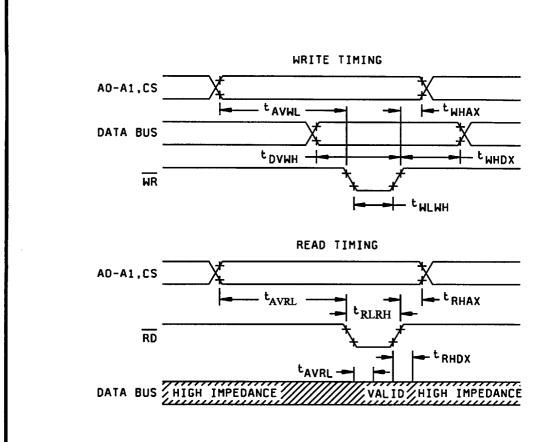
FIGURE 4. Timing waveforms. - Contined
