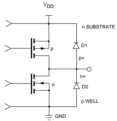
Fig. 2b Equivalent Output Circuit
