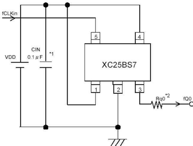
\*1: C<sub>IN</sub> (by-pass capacitor, 0.1 µF) should be connected to the IC as close as possible.
