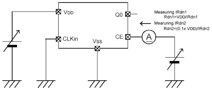
Output Off Leak Current
