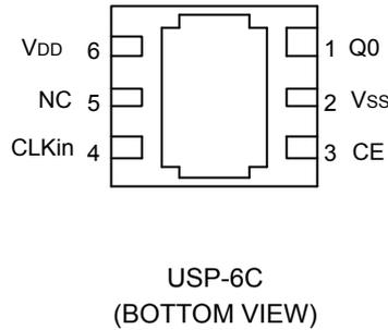
\* The dissipation pad (TAB) of the bottom view of the USP-6C package should be connected to the V<sub>SS</sub> (No. 2) pin.
