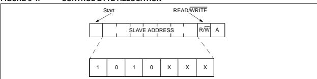
X = Don't care. B0 is don't care for DDC Monitor Port, but is used by the Microcontroller Access Port to select which of the two 256 word blocks of memory are to be accessed.
