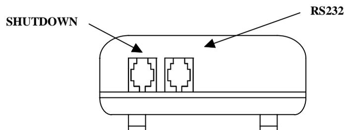
2.5.1 - RS232 connector (RJ11 type) with the following signals:
