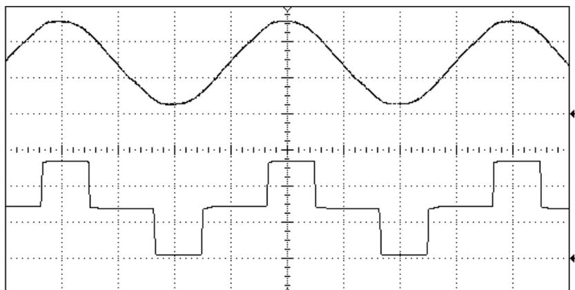
Output voltage waveform ( 2.- On mains )
