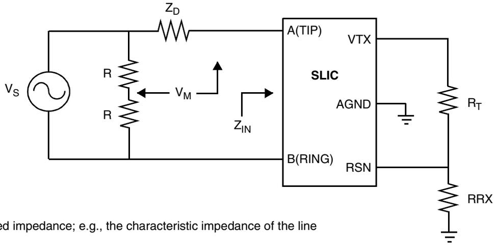
$Z_D$ : The desired impedance; e.g., the characteristic impedance of the line
