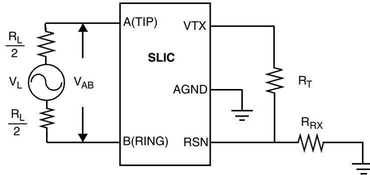
$$I_{L2-4} = 20 \log (V_{TX} / V_{AB})$$
