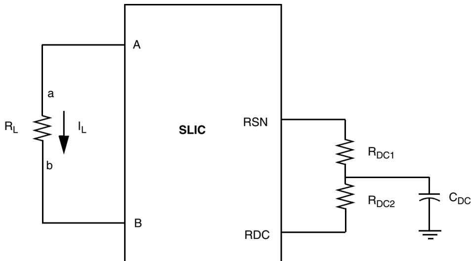
Feed current programmed by  $R_{DC1}$  and  $R_{DC2}$
