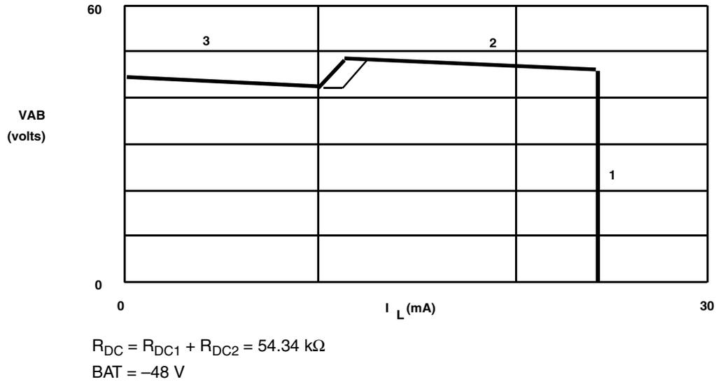
$$1. V_{AB} = I_L R_L' = \frac{1250}{RDC} R_L', \text{ where } R_L' = R_L + 2R_F$$
