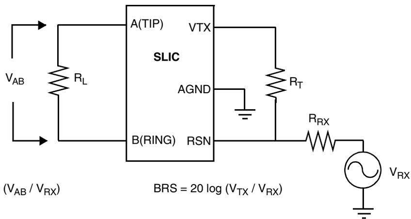
$$I_{L4-2} = 20 \log (V_{AB} / V_{RX})$$
