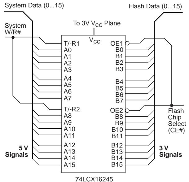
**Figure 3. Data Bus Transceiver**
