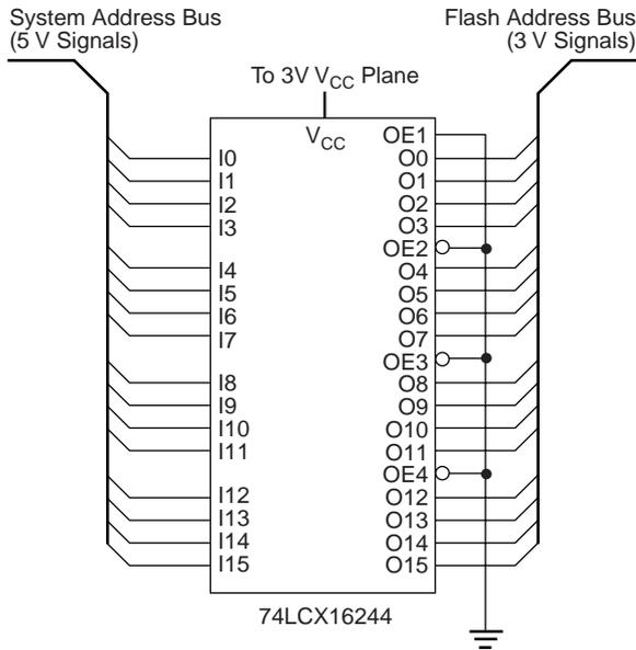
**Figure 1. Address Translation Circuitry (First 16 Address Lines)**
