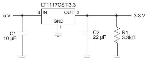
**Figure 6. Voltage Regulation Using Fixed Regulator IC**
