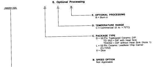
A. DEVICE NUMBER/DESCRIPTION Am29116 High-Performance 16-Bit MPU Am29116A
