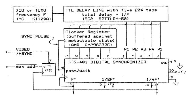
The RCS-401 generates three frequencies separated by binary factors. The highest of the three is equal to the input frequency (F) from the XCO. The lower two are 1/2F and 1/4F subharmonics. Each of the three output signals is phase-locked to the sync pulse, and all cycles are whole and well-defined with respect to the active edge of the sync pulse as shown by the timing diagram on the next page.
