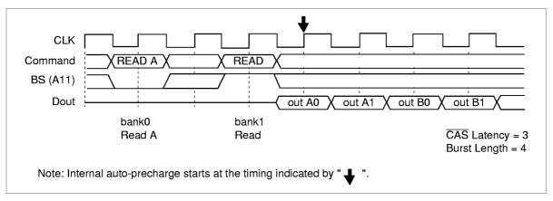
**Same bank:** The consecutive read command (the same bank) can not be executed. It is necessary to separate the two read commands with a bank active command.
