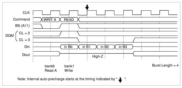
**Same bank:** The consecutive write command (the same bank) can not be executed. It is necessary to separate the two commands with a bank active command.
