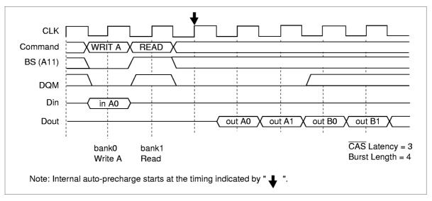
**Same bank:** The consecutive read command (the same bank) can not be executed. It is necessary to separate the two commands with a bank active command.
