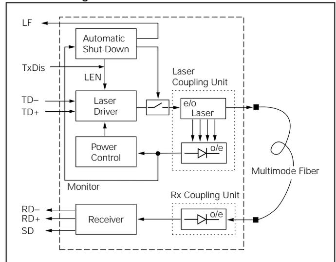
The receiver component converts the optical serial data into PECL compatible electrical data (RD+ and RD-). The Signal Detect (SD, active high) shows whether an optical signal is present.
