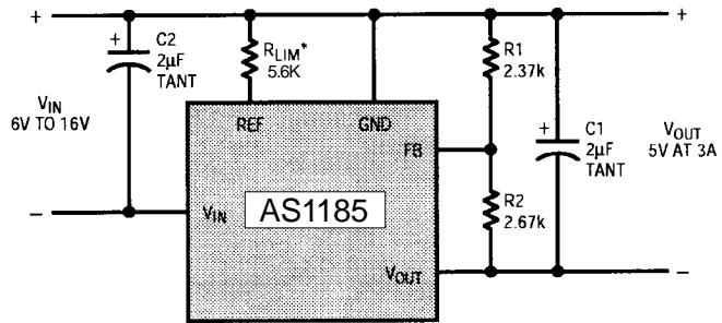
\*CURRENT LIMIT =  $15\text{k}/R_{\text{LIM}} = 2.7\text{A}$
