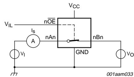
V<sub>I</sub> = V<sub>CC</sub> or GND and V<sub>O</sub> = open circuit.
