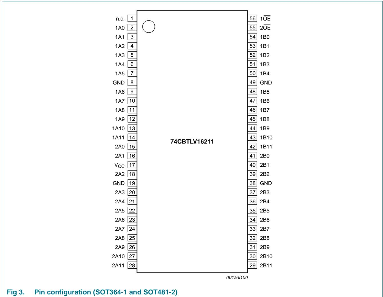
Fig 3. Pin configuration (SOT364-1 and SOT481-2)
