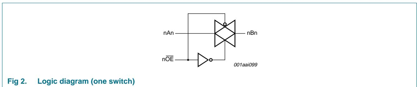
Fig 2. Logic diagram (one switch)
