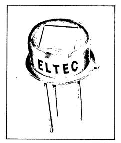
**Model 5192** consists of two physically separate lithium tantalate sensing elements and a FET source follower sealed into a standard TO-5 housing with an optical filter.
