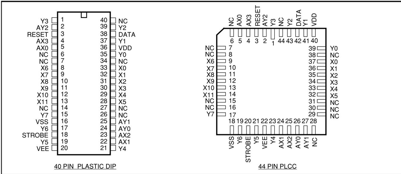
Figure 2 - Pin Connections
