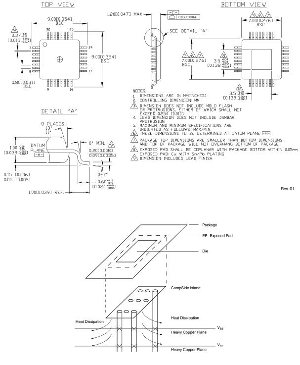
PCB Thermal Consideration for 32-Pin EPAD-TQFP Package
