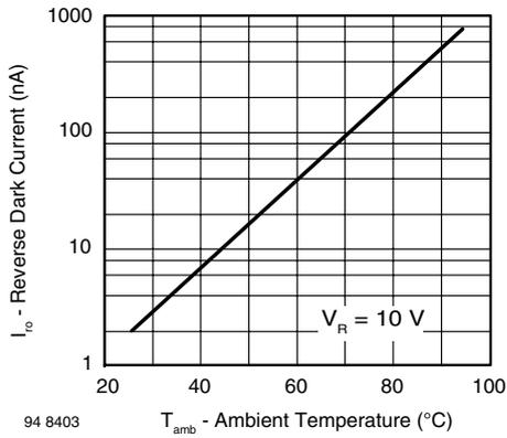
Figure 1. Reverse Dark Current vs. Ambient Temperature
