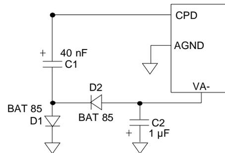
**Figure 4. Generating VA- with a Charge Pump**
