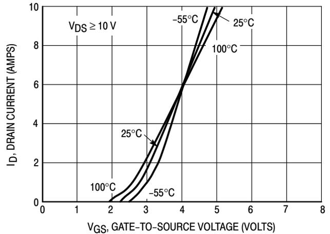
Figure 2. Transfer Characteristics
