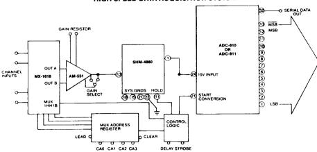
The four DATEL components shown in the diagram make up a 12-bit, high-speed data acquisition system capable of throughput rates of 200 kHz. The system can accept up to 16 single-ended input channels using DATEL's MX-1616 CMOS multiplexer or up to eight differential channels using the MX-908.
