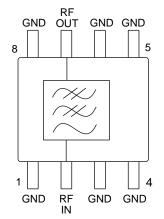
All unused pins must be RF and DC grounded. Pins 1 and 4 are thermal ground contacts.
