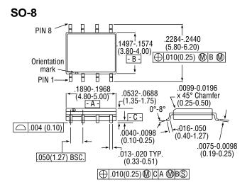
$\begin{array}{l} \mbox{8- Lead SOP outline dimensions} \\ \mbox{Narrow body .150} \\ \mbox{(All dimensions per JEDEC No. MS-012-AA, Issue C)} \\ \mbox{Dimensions in ( ) are in mm.} \\ \mbox{Unless Otherwise Noted: .xxx = \pm0.010 (.xx = \pm0.25)} \\ \mbox{.xx = \pm0.02 (.x = \pm0.5)} \end{array}$
