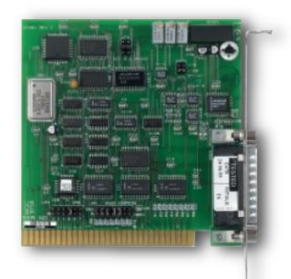
Timer 2: Resolution (Cascade from TIMER 1)  $1\mu$ S Minimum Time Interval:  $2\mu$ S Maximum Time Interval: 65.535mS
