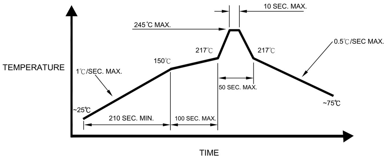
The reflow temperature 240°C~245°C is recommended and the soldering temperature should be not higher than 245°C (one time only)
