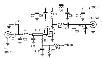
C1, C7,C8, C11 .047 uF 500V ceramic disc C2, C12 ARCO 465 75-380pF mica trimmer C3 2x 4700pF ATC 700B C4, C9-C10 8200pF 500V NPO ceramic C5 200 pF ATC 100E C6 150 pF ATC 700B L1 90 nH 4t #18 0.25"d .25" I L2 200 nH - 3t #8 1" dia 1" I L3 6 uH - 22t #24 enam. 0.5" dia. L4 500 nH 2t on 850u .5" bead R1-R3 1k  $\Omega$  1/4W TL1 .112" x 1 " (50  $\Omega$ ) Stripline
