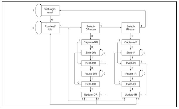
Note: The value adjacent to each state transition in this figure represents the signal present at TMS at the time of a rising edge at TCK.
