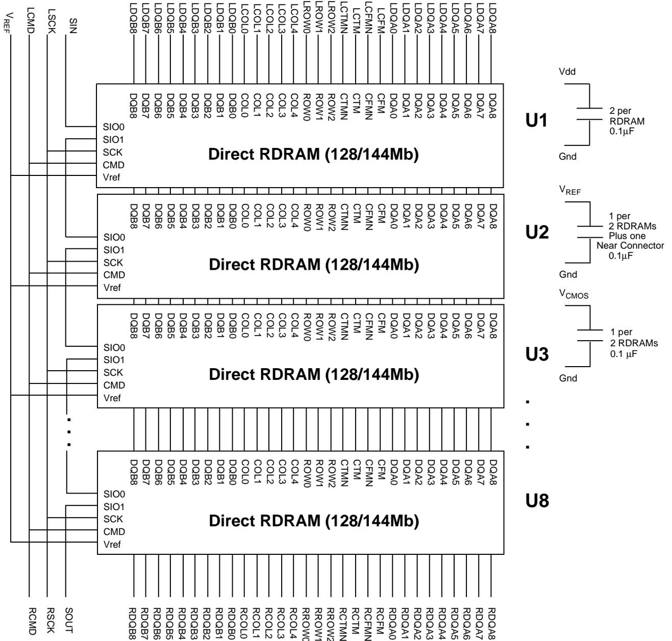
Note 1: Rambus Channel signals form a loop through the RIMM module, with the exception of the SIO chain.
