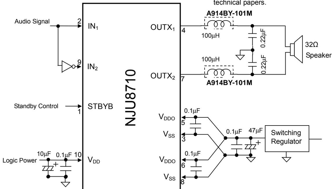
Note 4) De-coupling capacitors must be connected between each power supply terminal and GND terminal.
