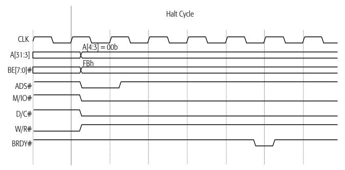
Figure 77. Basic Special Bus Cycle (Halt Cycle)
