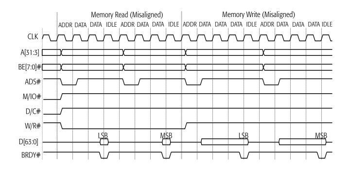
Figure 61. Misaligned Single-Transfer Memory Read and Write
