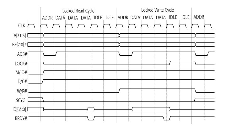
Figure 74. Basic Locked Operation
