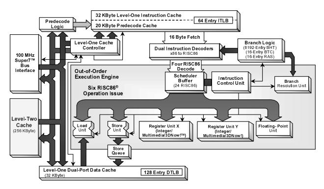
Figure 1. AMD-K6<sup>™</sup>-IIIE+ Processor Block Diagram
