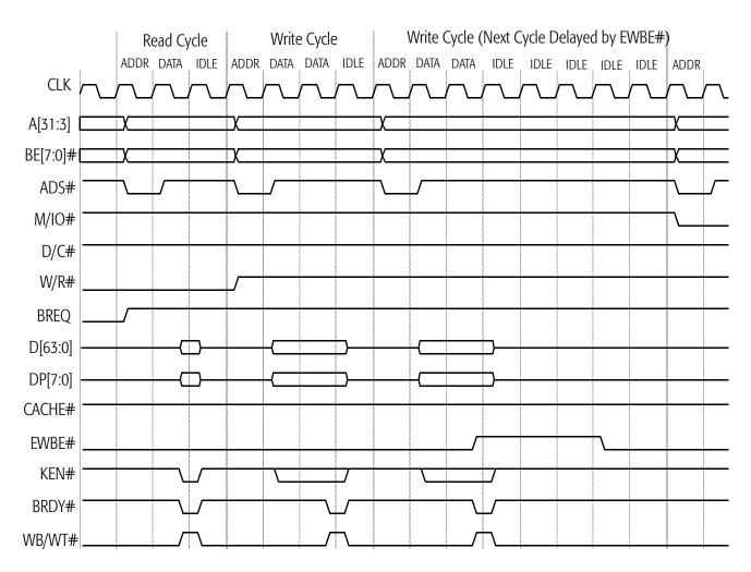
Figure 60. Non-Pipelined Single-Transfer Memory Read/Write and Write Delayed by EWBE#
