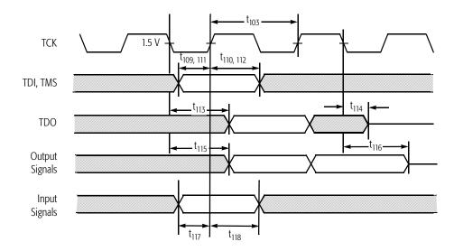
Figure 112. Test Signal Timing Diagram
