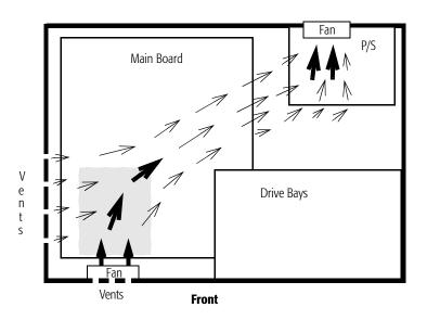
Figure 119. Airflow Path in a Dual-Fan System
