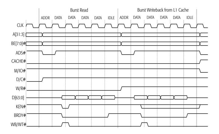
Figure 63. Burst Writeback due to Cache-Line Replacement
