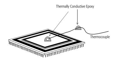
Figure 116. Measuring Case Temperature
