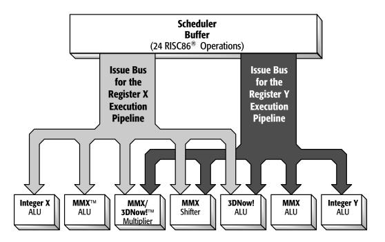
Figure 6. Register X and Y Pipeline Functional Units
