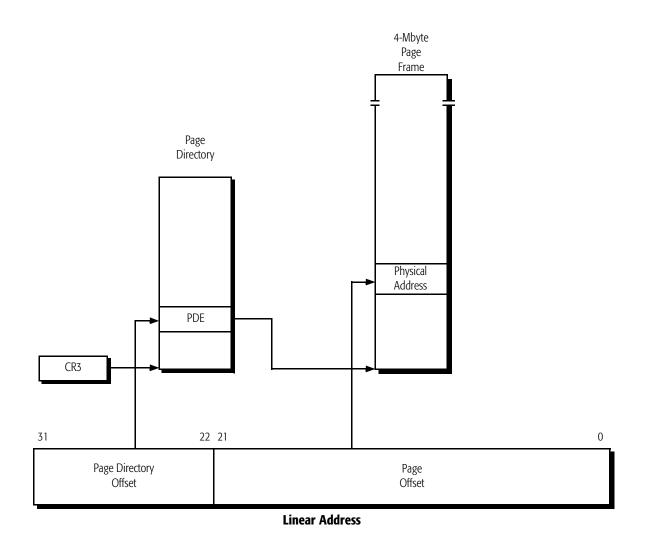
Figure 47. 4-Mbyte Paging Mechanism
