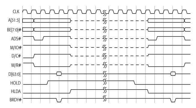
Figure 66. Basic HOLD/HLDA Operation
