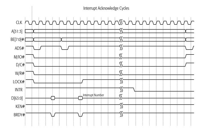
Figure 76. Interrupt Acknowledge Operation
