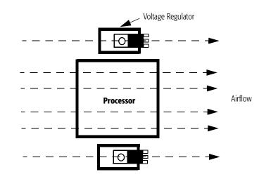
Figure 117. Voltage Regulator Placement
