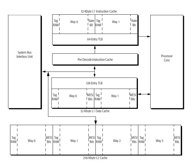
Figure 82. L1 and L2 Cache Organization for the AMD-K6<sup>™</sup>-IIIE+ Processor
