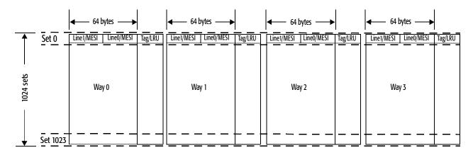
Figure 91. L2 Cache Organization for AMD-K6<sup>™</sup>-IIIE+ Processor
