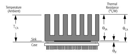
Figure 113. Thermal Model (CPGA Package)
