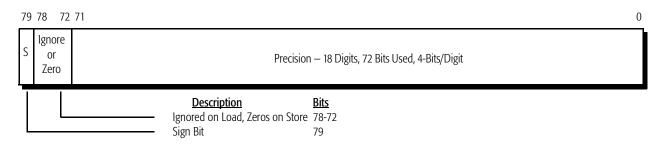
Figure 15. Packed Decimal Data Register
