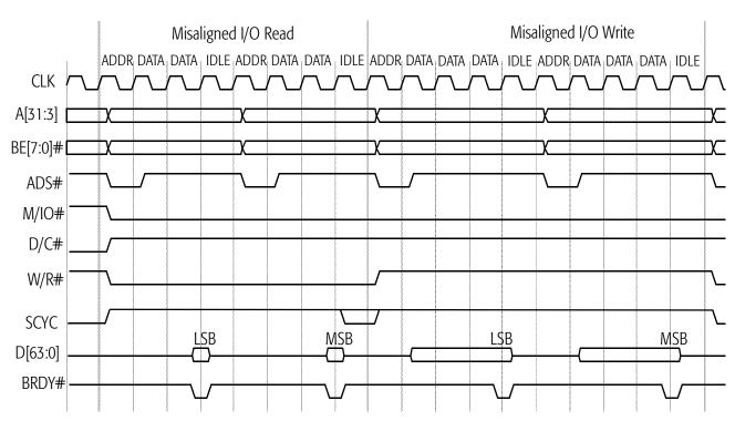
Figure 65. Misaligned I/O Transfer
