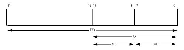
Figure 7. EAX Register with 16-Bit and 8-Bit Name Components
