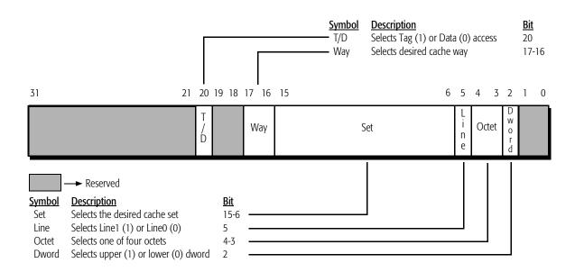
Figure 93. L2 Tag or Data Location for the AMD-K6<sup>™</sup>-IIIE+ Processor–EDX
