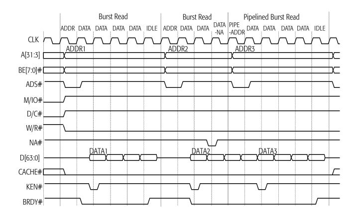
Figure 62. Burst Reads and Pipelined Burst Reads
