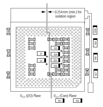
Figure 103. Suggested Component Placement for CPGA Package
