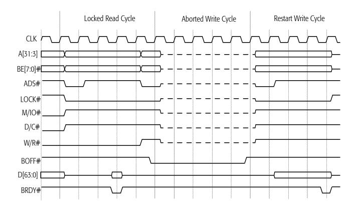
Figure 75. Locked Operation with BOFF# Intervention
