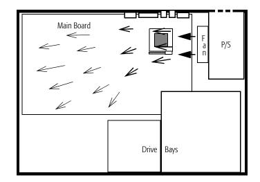
Figure 120. Airflow Path in an ATX Form-Factor System
