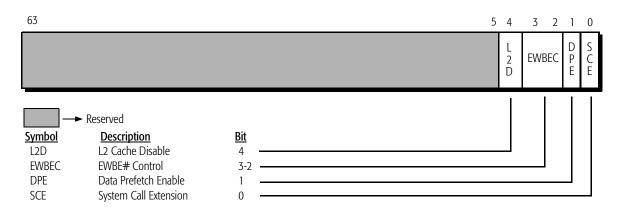
Figure 34. Extended Feature Enable Register (EFER)
