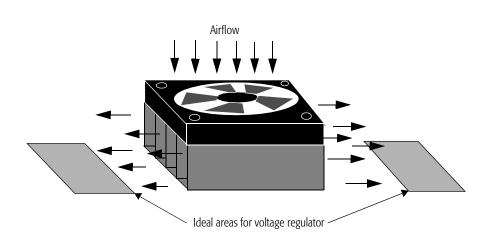
Figure 118. Airflow for a Heatsink with Fan
