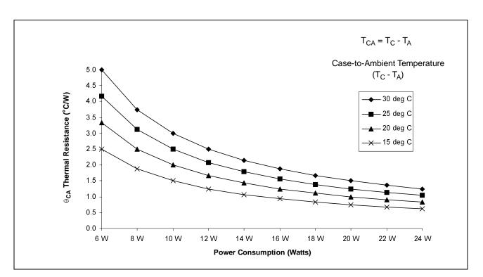
Figure 114. Power Consumption and Thermal Resistance (CPGA Package)
