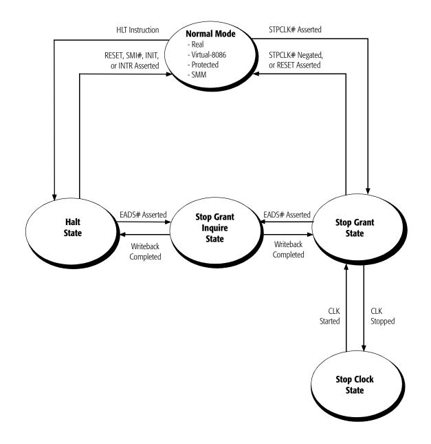
Figure 101. Clock Control State Transitions for Standard-Power Versions of the AMD-K6<sup>™</sup>-IIIE+ Processor
