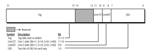
Figure 95. L2 Tag Information for the AMD-K6<sup>™</sup>-IIIE+ Processor–EAX
