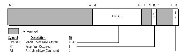
Figure 86. Page Flush/Invalidate Register (PFIR)
