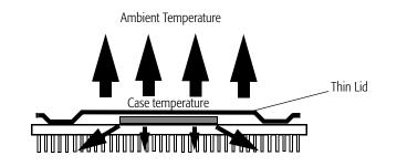
Figure 115. Processor Heat Dissipation Path
