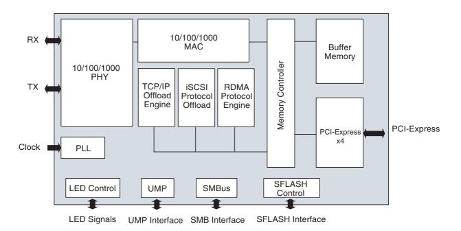
The **BCM5708C** provides a fully integrated Layer 4 and Layer 5 solution - TCP/IP, RDMA and iSCSI 1.0/iSER along with a complete 10/100/1000BASE-T Gigabit Ethernet, IEEE 802.3 compliant Media Access Control (MAC) and Physical Layer Transceiver solution for high performance network applications. By itself, the **BCM5708C** provides a complete single-chip Gigabit Ethernet NIC with a TCP/IP Offload Engine, RDMA NIC (RNIC), iSCSI 1.0/iSER HBA or LOM solution.
