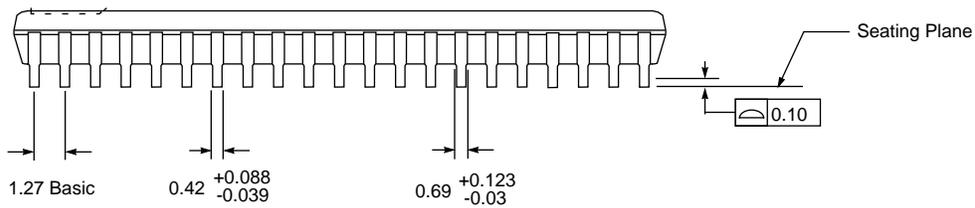
**NOTE:** All dimensions are in millimeters; Package diagrams are not drawn to scale.
