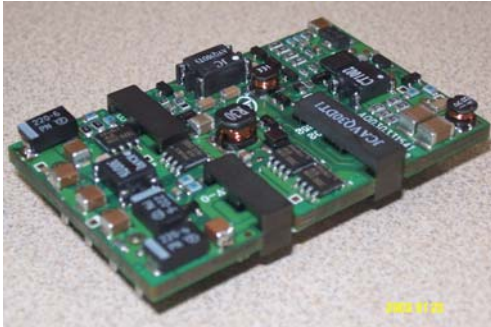
Industry Standard Size: 2.28"X 1.45" X 0.43"package
