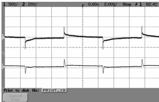
ALQ07FM 25%-50%-25% I_{o2,nom} ( I_{o2} ) load change, I_{o1} = 50\%I_{o1,nom} (ch1: V_{o1} ,ch2: V_{o2} )
