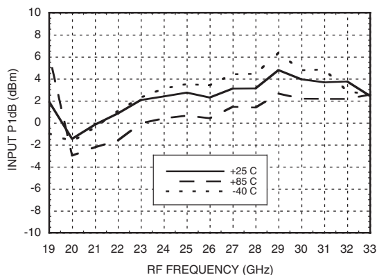
Input P1dB vs. Temperature @ LO = -4 dBm, Vdd = +4V
