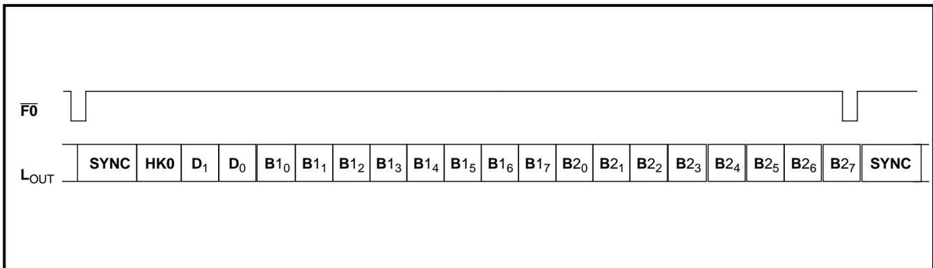
Figure 12 - Frame Format - 160 kbit/s (Modes 0, 2, 3, 4, 6)
