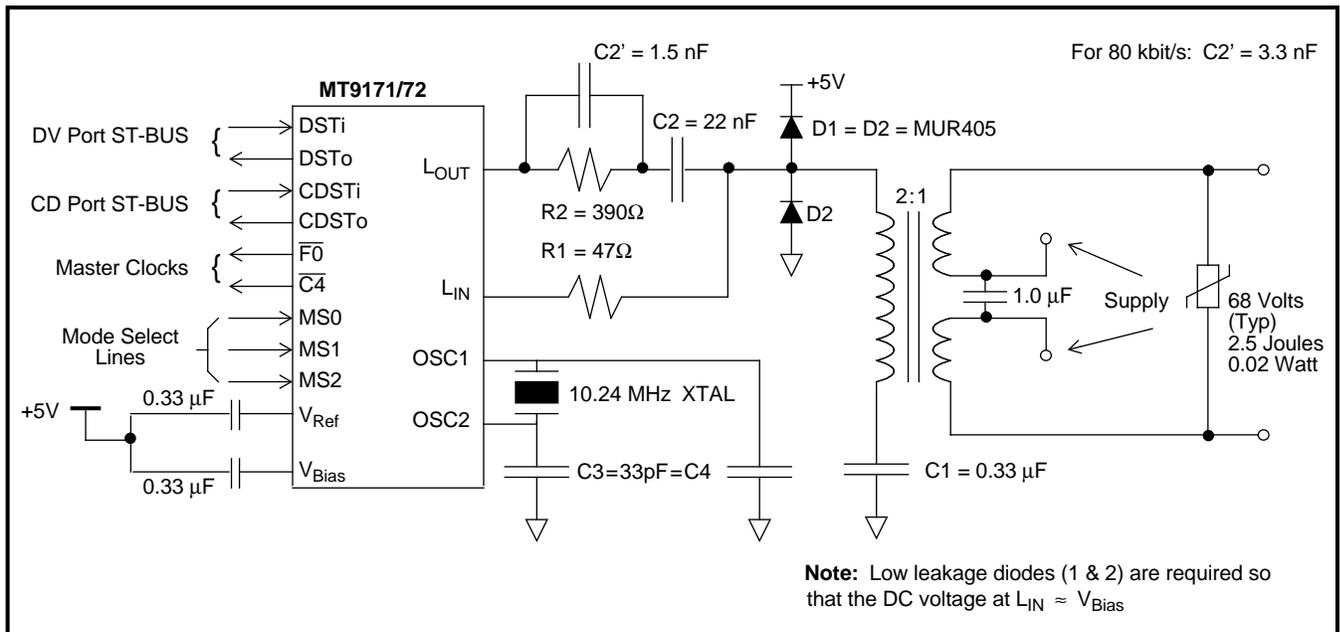
Figure 14 - Typical Connection Diagram - SLV/DN Mode, 160 kbit/s
