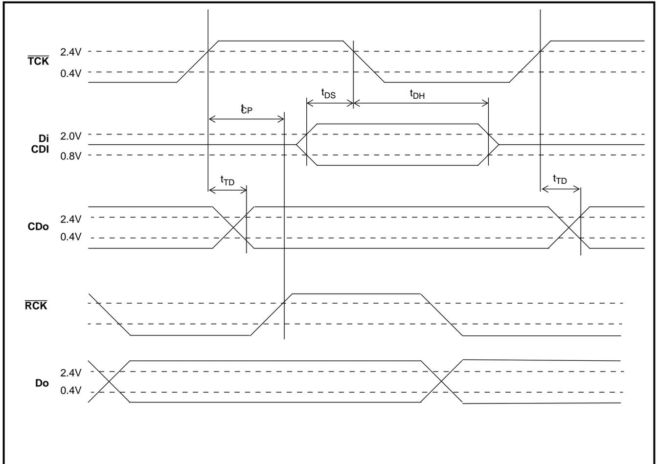
Figure 21 - Data Timing for Slave Modem Mode
