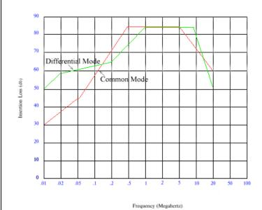
The 1135 Series is designed to provide filtering for DC systems operating in very noisy environments. This filter series will attenuate RF noise from switching power supplies as well as transient noise from relays and other switching devices.
