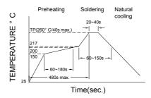
Figure 1. Re-flow Soldering
