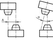
Parallel displacement Angle displacement  $A \le 8 \text{ mm}$
