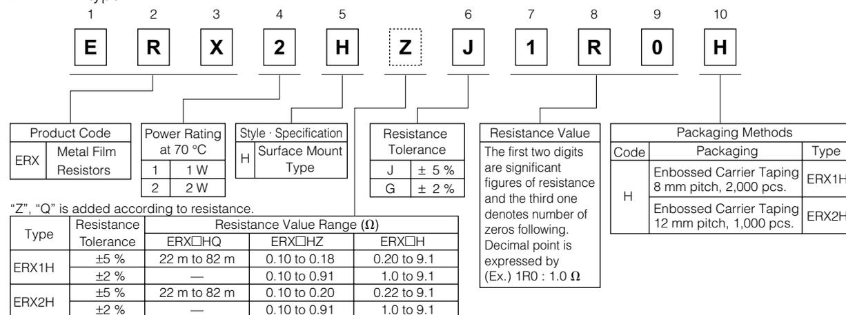
The above example 1 shows a metal film resistor SMD type, 2 W power rating, resistance value of 1.0 Ω, tolerance ±5 %, and embossed taping.
