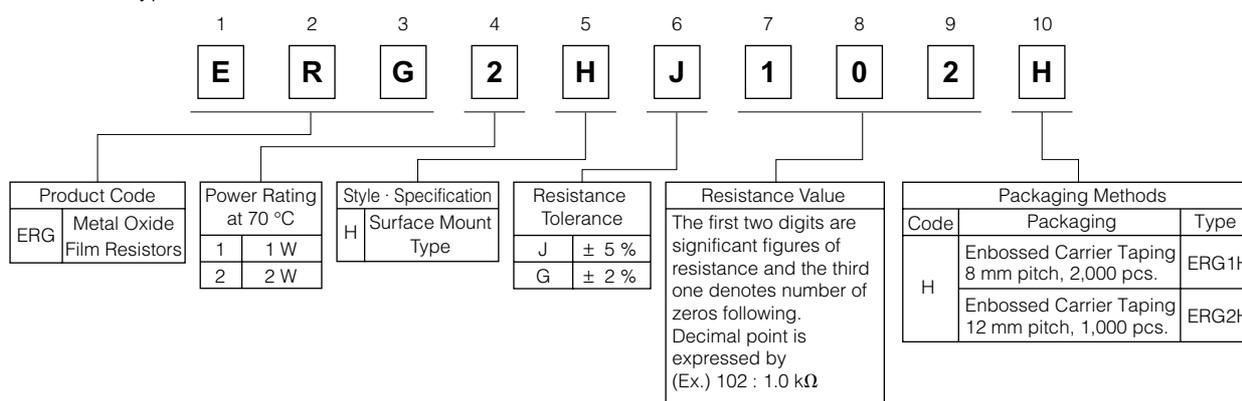
The above example 2 shows a metal oxide film resistor SMD type, 2 W power rating, resistance value of 1.0 kΩ, tolerance ±5 %, and embossed taping.
