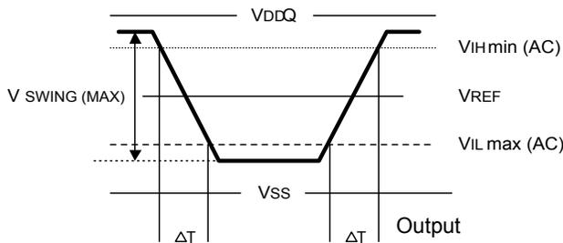
$$\text{SLEW} = (V_{IHmin} (AC) - V_{Lmax} (AC)) / \Delta T$$
