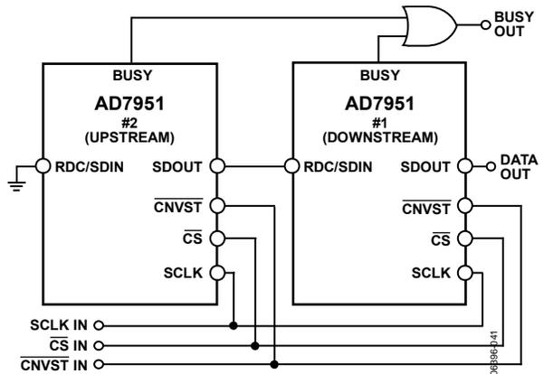
Figure 41. Two AD7951 Devices in a Daisy-Chain Configuration
