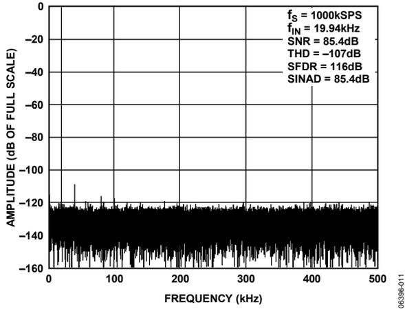
Figure 11. FFT 20 kHz
