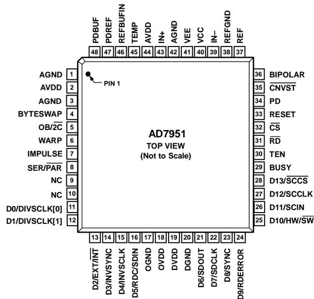
Figure 4. Pin Configuration
