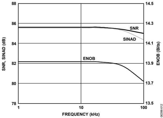
Figure 12. SNR, SINAD, and ENOB vs. Frequency
