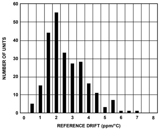
Figure 19. Reference Voltage Temperature Coefficient Distribution (247 Devices)
