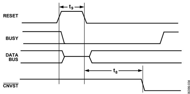
Figure 34. RESET Timing
