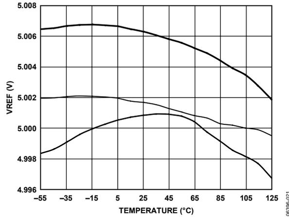
Figure 21. Typical Reference Voltage Output vs. Temperature (3 Devices)
