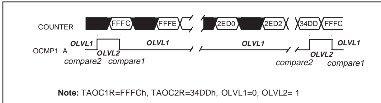
Figure 2. 0% duty cycle minimum value with OC1R=FFFCh=Counter Reset Value
